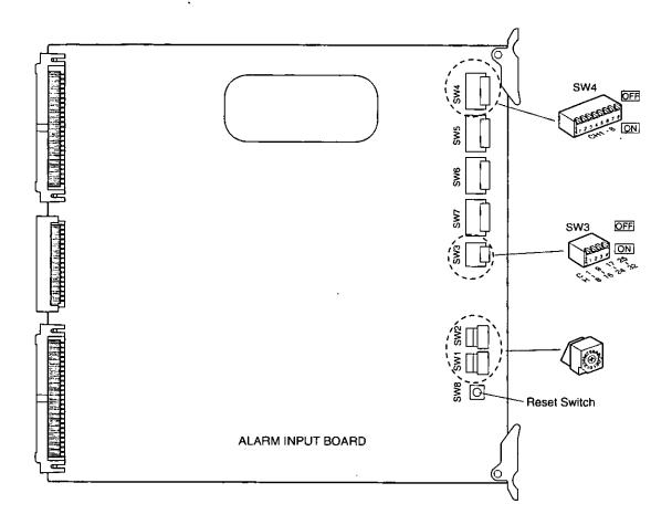
1. Set switches (SW1 and SW2) on the board to designate the Alarm Input board number as shown in the following table. The factory default setting is Board Number 1 (00).
